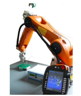
Special Iron unit and feeder designed for KUKA - ALNEA Zeus Controller
